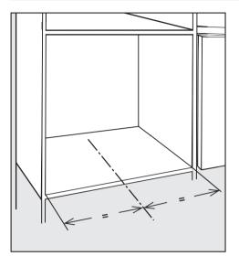
Draw a line inside the housing unit to mark the middle of the unit as illustrated.
